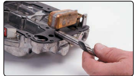
Checking float level with a 7/16" drill bit
