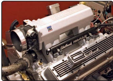
An Edelbrock Pro-Flo XT EFI System being tested on our SuperFlow Dyno
