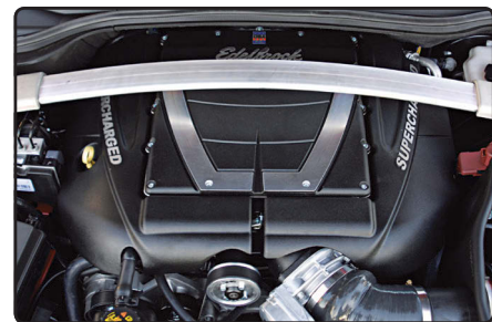
E-Force Supercharger Systems #1563 with low profile top to accommodate the vent on the factory hood.
